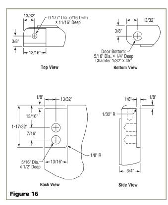
Route notch in top corner of overlay panel as shown (see Top and Side Views). Top of notch is entire depth of panel, front to back.
